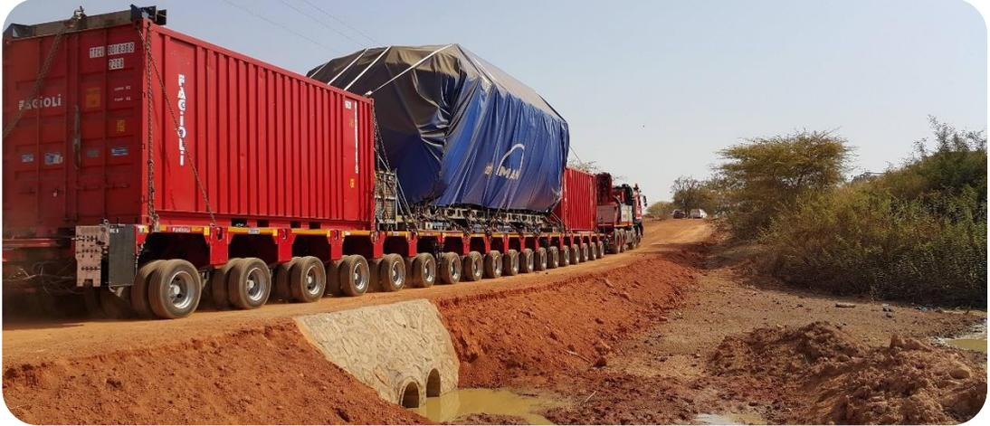
Fagioli were contracted for the transport of 4 engines weighing 256 ton each from Tema port (Ghana) to Niamey power plant (Niger) for a total of 1550 km for each trip. -Offloading of no. 4 engines type at Tema port (Ghana) from vessel onto 18 axles modular trailers and storage operations in the port area.
