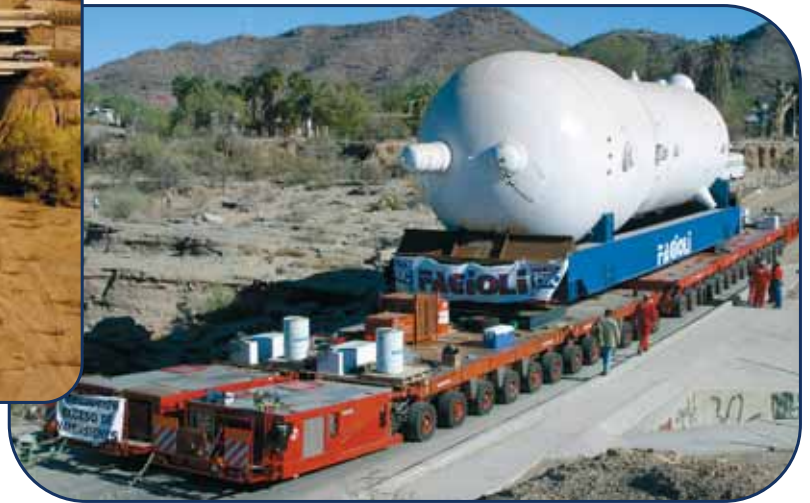
TRANSPORT OF 2 STEAM GENERATORS X 750 TONS FROM MILAN TO NUCLEAR POWER PLANT ARIZONA USA, 2003
